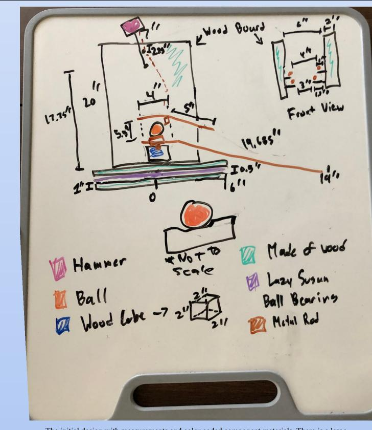
The initial design with measurements and color coded component materials. There is a large cross-section looking through the right support plank and into the central mechanism. On the top right, there is a view of the front without the hammer to show the measurements of the rails that will guide the ball. Also shown is the basic design developed to hold the ball in place before it is struck by the
