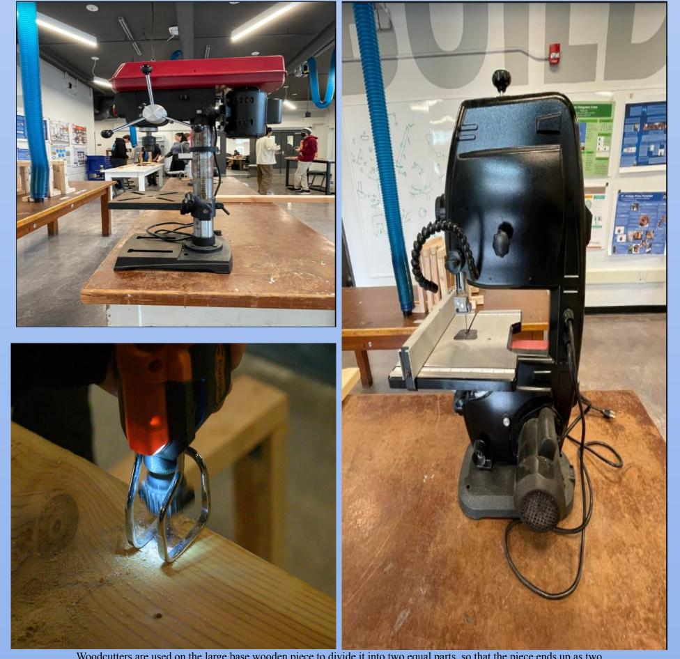
Woodcutters are used on the large base wooden piece to divide it into two equal parts, so that the piece ends up as two flat planks. A saw is then used to actually cut the piece. Afterwards, the tape measure and marker are used to mark where the two base planks should be drilled. A drill is then used to actually drill the holes. Finally, a screwdriver is used to secure the lazy susan in between the two wood planks, and a level is used to make sure the base is level.
